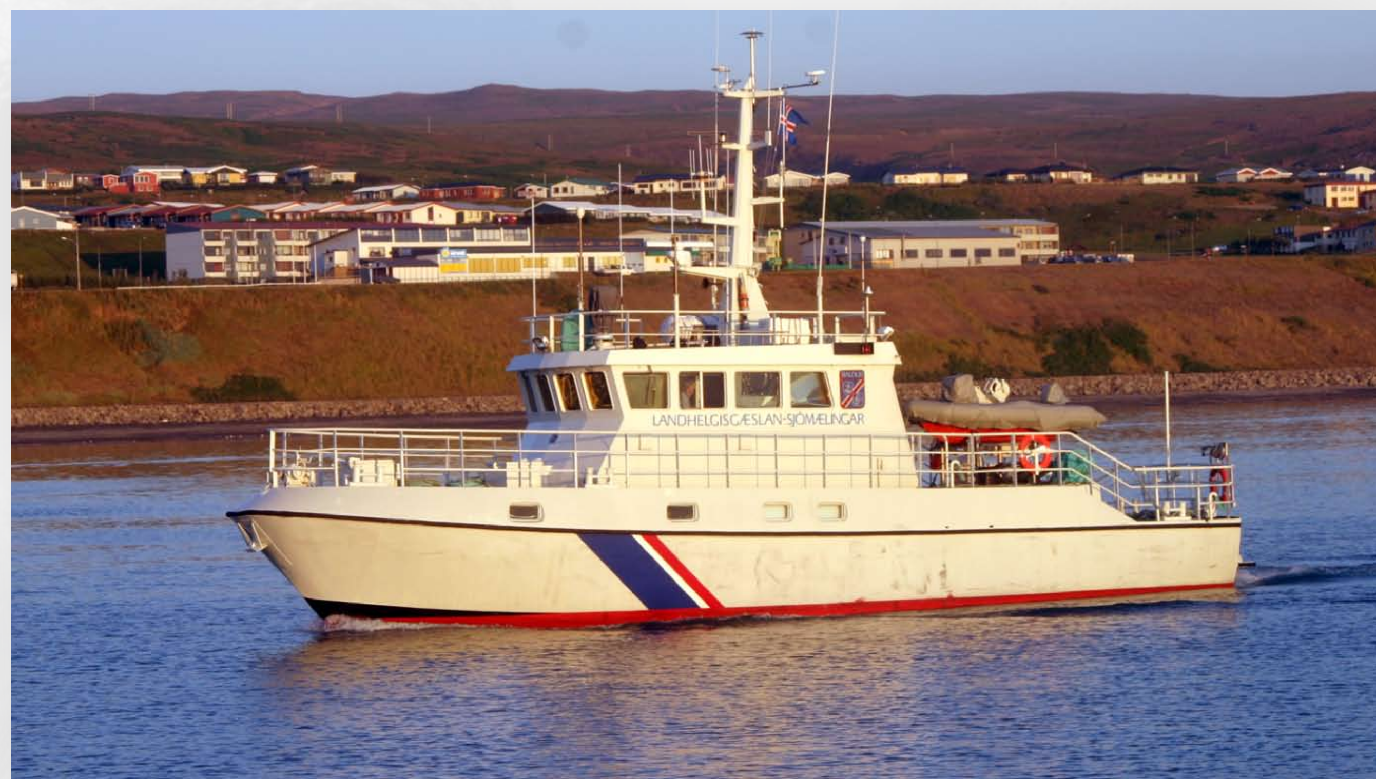
M/V Baldur was built as a custom survey vessel for the Icelandic Coast Guard – Hydrographic Department in 1991. The vessel is 21 meters long, 5 meters wide and is fitted with RESON multibeam echo sounder
