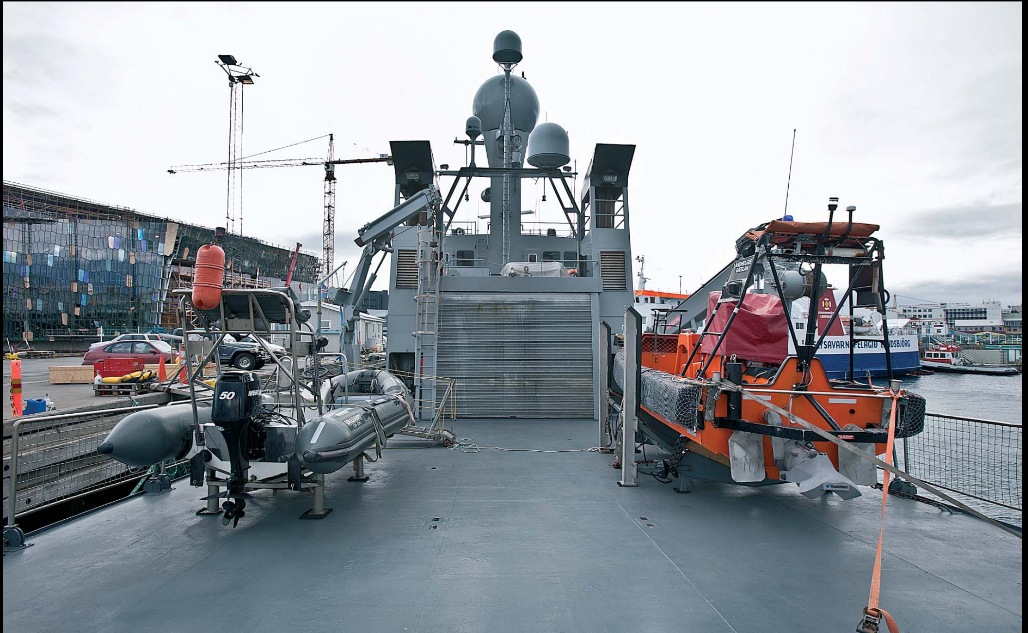
Two Davits (deck cranes) are available for launching and recovery of boarding boats.
